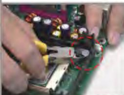
This image shows the retention module with all four push-pins removed.
